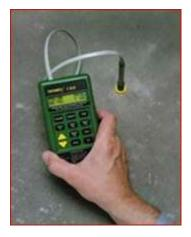
Tramex Surface Moisture Meter Tramex Inserted Probe Moisture Meter
