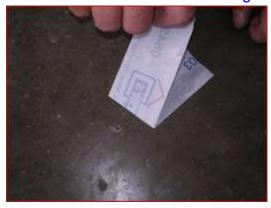
Cross Hatch Test - No visible cuts or flaking on the back of the tape
