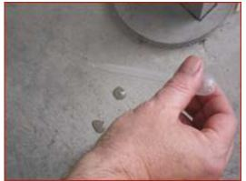
Water Droplet: Pipette Application Note the immediate absorption
